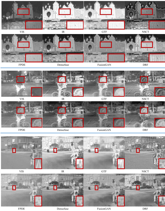
Fig. 8. Qualitative comparison of our DRF with five state-of-the-art methods on three typical VIS-IR image pairs in the RoadScene data set. In each group of results, from top to bottom (from left to right): visible and infrared image pair, fusion results of GTF [16], NSCT [40], FPDE [41], Densefuse [42], FusionGAN [18], and our DRF.
