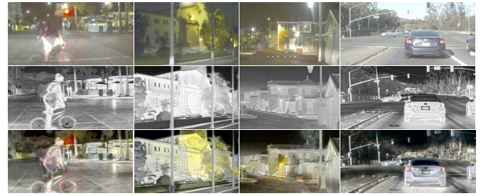
Fig. 9. Qualitative fusion results on the four image pairs in the RoadScene data set. From top to bottom: the RGB VIS images, the gray IR images, and the RGB fusion results.
