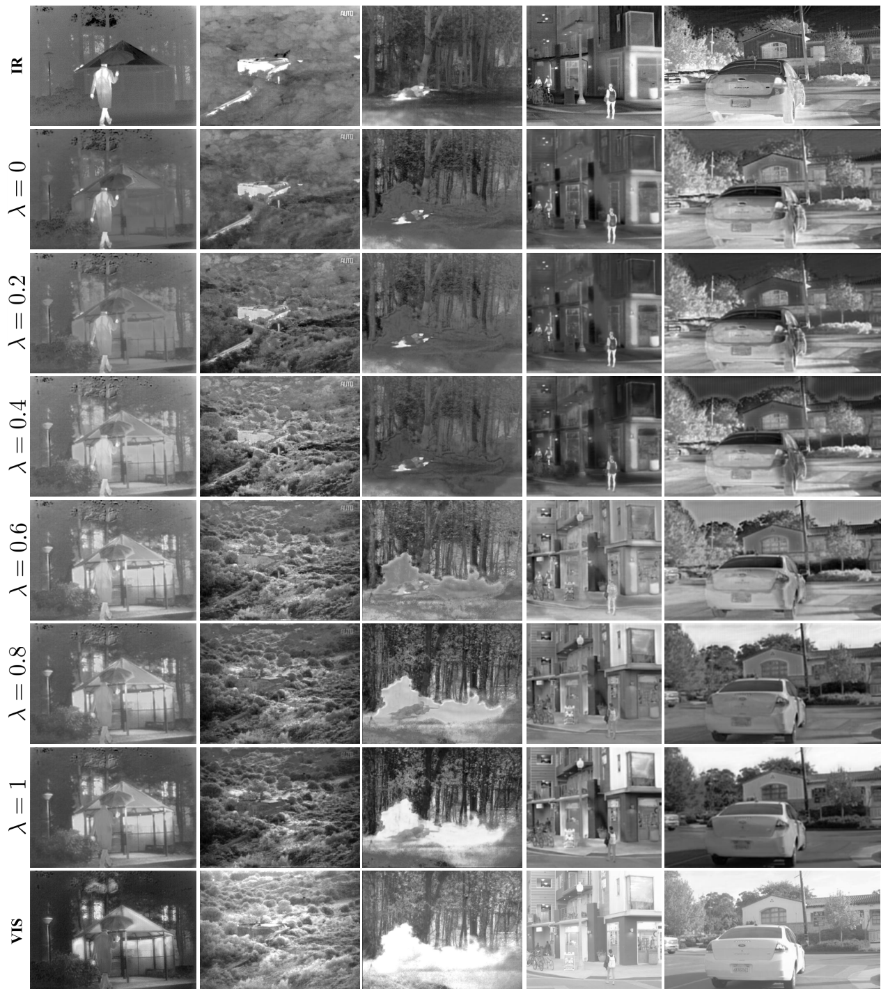
Fig. 10. Qualitative fusion results on the five image pairs (the first three image pairs are from the TNO data set, and the last two image pairs are from the RoadScene data set). From top to bottom: infrared image, fusion results when \lambda = 0, 0.2, 0.4, 0.6, 0.8, 1 , and visible image.
